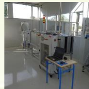
Single flow configuration: Filtration, Cooling, Heating, Blowing, Humidification
