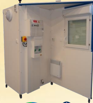
EnOcean Smart Home – Home automation wiring and installation in a full-scale 3D structure
