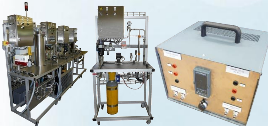
Regulflex – Modular didactic production line of carbonated drinks to study process control and associated instrumentation
