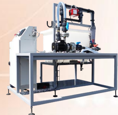
ErmaPompes – Study, maintenance and testing bench for industrial pumps
