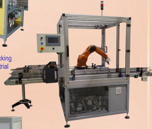
Polyprod - Multi-format packaging (filling, dosing and capping of liquids and pellets in jars and bottles)
