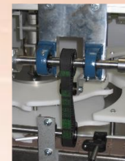
Pulley alignment (worm screw rotation)
