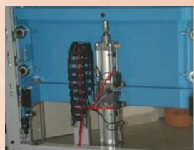
2 double-acting cylinders connected in tandem
