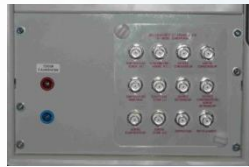
Measuring console for voltage, temperature and hygrometry
