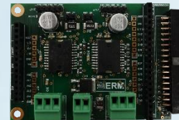
Controller board for brushless / stepper / DC motors
