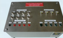
DI15 Acquisition and control unit with NI 6009 input/output cards
