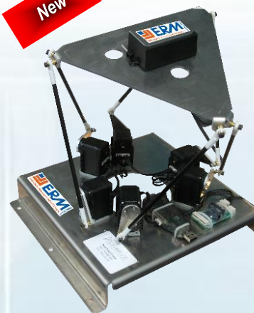
6-axis certification test bench for inertial measurement unit
