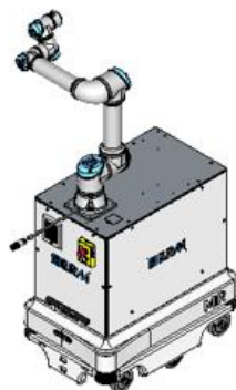
AGV MiR100 with UR eSeries collaborative arm
