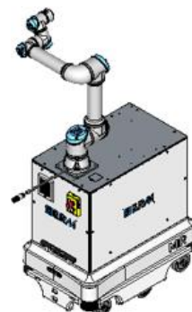
AGV MiR100 with UR eSeries collaborative arm
