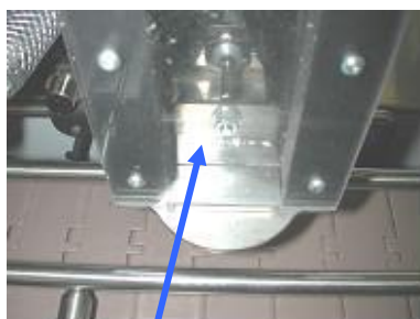
Cylinder "solid product outlet shutter".
