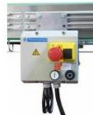
Starter box (Integrated on CE50)
