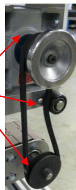
Replacement of the chain sprocket transmission with a V-belt pulley
