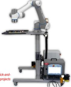
Cobot Dobot station with vision and parts for 2D and pick-andplace uncoiling projects
