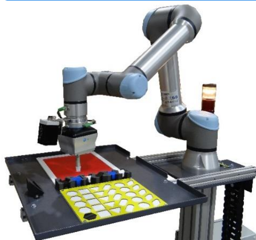
Cobot & Vision UR5 eSeries station with parts for 2D and pick-and-place projects
