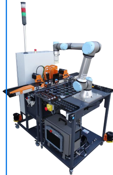
Collaborative Capping & Assembly Robot (Universal Robots UR5 eSeries)
