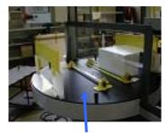
Manual turntable for loading and unloading cartons.
