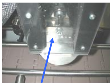
Cylinder "solid product outlet shutter".
