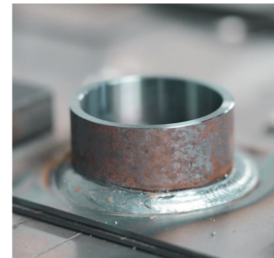
Arc welding: Carbon steel
