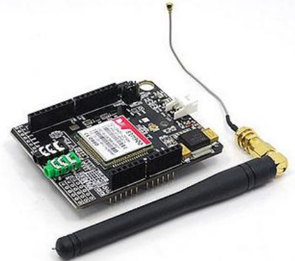
Figure 16 - PR15 Module de communication GSM
