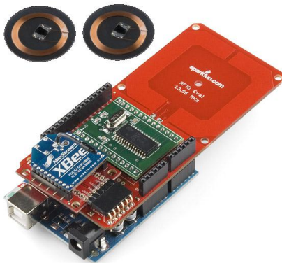
Figure 17 - PR16 Kit de communication RFID
