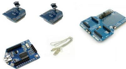
Figure 18 - PR17 Kit de communication RF 868MHz
