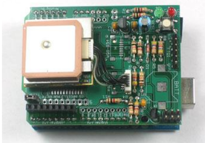
Figure 20 - PR20 Kit de communication GPS
