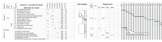
Range with, for each workstation, the breakdown of times by category and a diagram of movements on the workstation, then a time simulation graph (highlighting imbalances and NVA).
