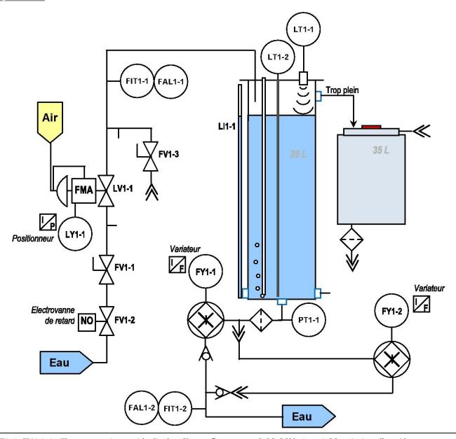
FIT1-1 /FAL1-1: Flow transmitter with display (Rotor flow meter 0,08-20l/min - 4-20 mA signal) + Alarm contact for "low" flow detection (24Vdc digital signal)
